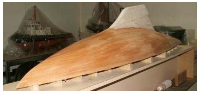
The finished hull weighs 11 kg, 8 of them in the keel.
