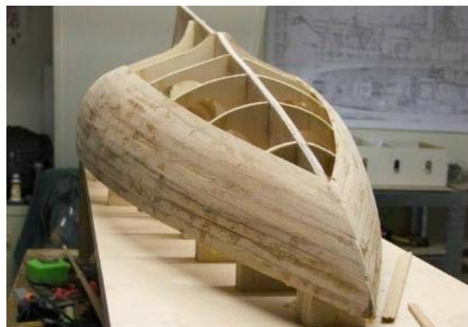
The planks are tapered and hand bent till the glue set, often with fingers attached!
